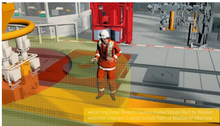
Personnel safety sensors may issue a visual, auditory, and/or tactile alert in response to a breach of the Warning Zone.
